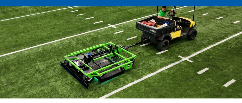
The GreenZapr disinfects synthetic turf surfaces with powerful germicidal UVC lights. Harmful micro-organisms such as MRSA, HIV, and influenza are eradicated through DNA destruction, eliminating the potential for "Super Bugs". Reliable on-board power via generator or optional rechargeable gel cell batteries provide the most efficient, cost-effective sanitation method available in the industry.
