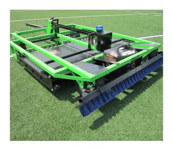
The GreenZapr is built with the same high-quality fabrication people have grown to expect from GreensGroomer. Powered by a portable Honda generator or optional rechargeable gel cell, the UVC lamps are mated into two reflector modules. The standard 3-pass treatment places over 7,800µW/cm² of UVC energy on any given portion of the field — killing all harmful micro-organisms.
